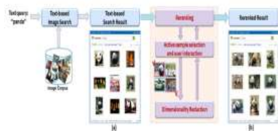
Fig: Framework for active re-ranking in web image search with the query "panda"
